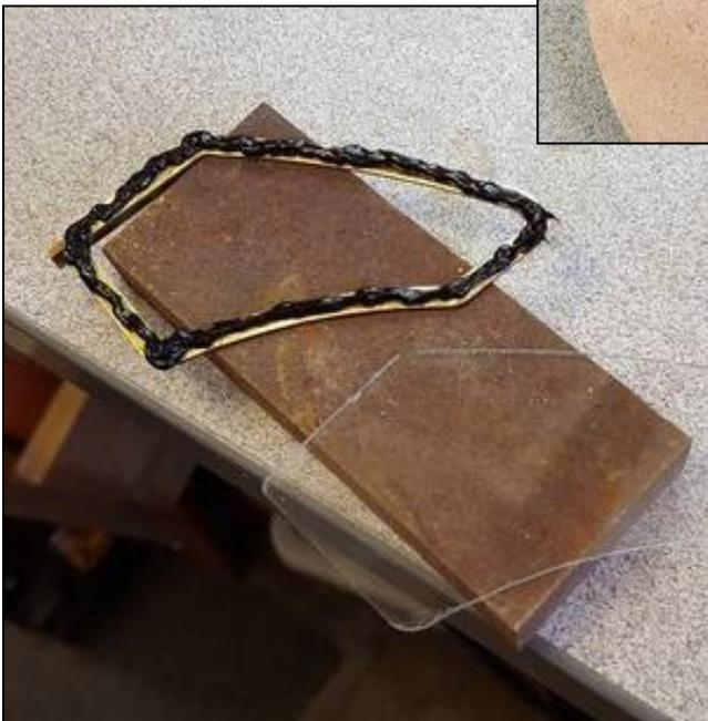
For this I have used a black RTV silicone which when cured will look very much like the rubber seal on the full size, RTV is used as it will stick with a strong bond to both the brass frame and glass window, it can also withstand very high heat. It can if needed, also be easily cut away with a sharp scalpel. BTW the slides are 3"x 2"x 1 mm thick
