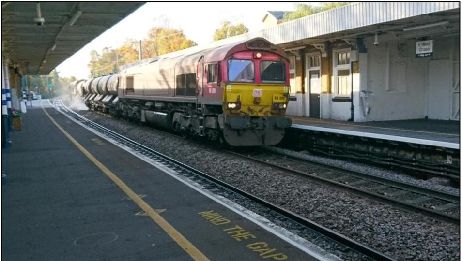
One of a fleet of 29 Network Rail locomotive hauled rail head treatment trains at Enfield Chase Station.
