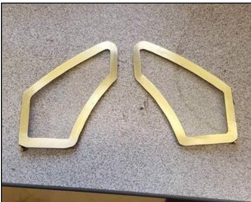
small amount of brass to be seen through the opening in the spectacle plate opening when fitted, approx. 0.75 mm wide band.
