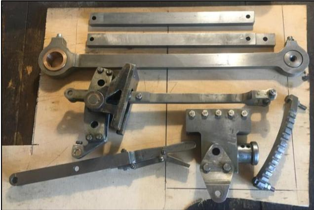
With so much of the engine dismantled and now in bits it was considered sensible to continue with the strip down take the opportunity to refurbish or repair as the engine was being rebuilt.
